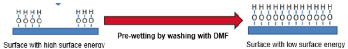
Figure 5.13: Reducing surface energy can enhance spreading of solution
